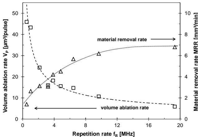
**Figure 12:** Volume ablation rate and material removal rate versus repetition rate obtained on stainless steel.
