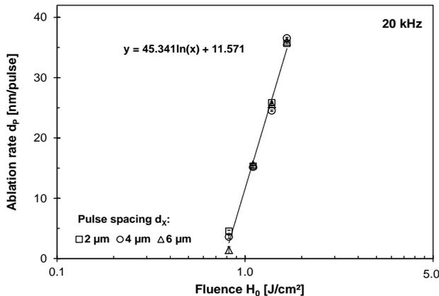
Figure 7: Ablation rate versus fluence obtained on zirconium oxide TZ-Black, the pulse spacing was varied.
