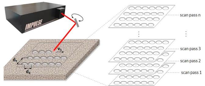
**Figure 5:** Schematic of the applied scan regime, where  $d_X$  is the pulse spacing,  $d_Y$  is the hatch distance,  $v_S$  is the scan speed, and  $n_S$  is the number of scan passes.
