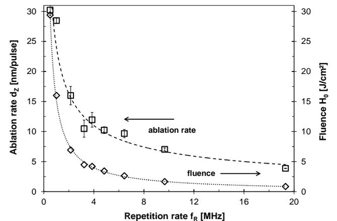
**Figure 11:** Ablation rate and fluence versus repetition rate obtained on stainless steel.
