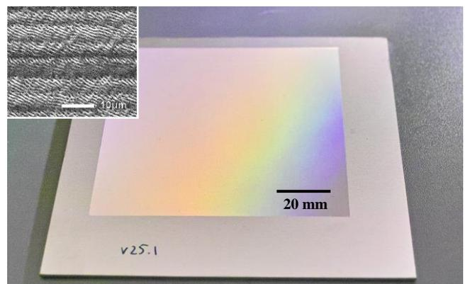
**Figure 14:** Rectangular diffraction pattern of 80 x 80 mm<sup>2</sup> (width x length) achieved on stainless steel, processing parameters were: 1.0 J/cm<sup>2</sup> fluence, 3.2 MHz repetition rate, 11.3 m/s scan speed, 5  $\mu\text{m}$  hatch distance and 1 scan pass.
