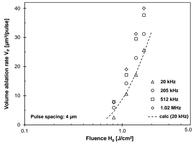
Figure 8: Volume ablation rate versus fluence obtained on zirconium oxide TZ-Black, the repetition rate was varied.
