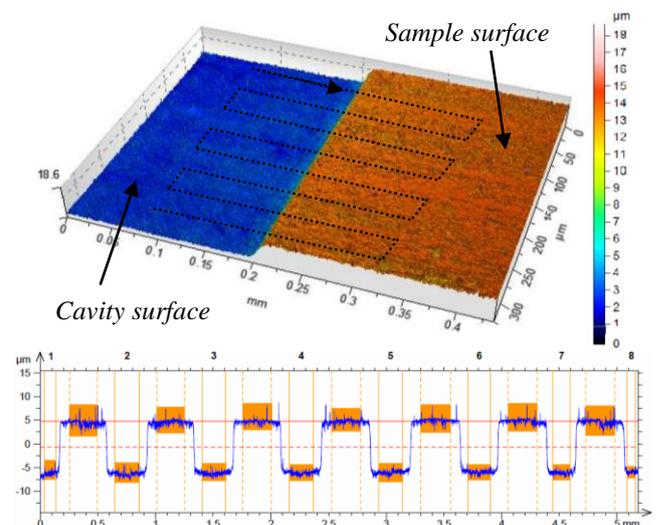
**Figure 6:** Laser processed cavity and depth profile.
