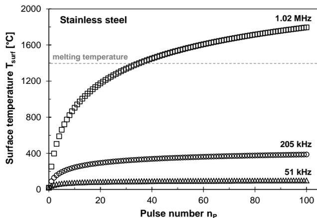
**Figure 2:** Surface temperature calculation on stainless steel, a thermal input of 3.5  $\mu\text{J}$  was taken into calculation, the repetition rate was varied between 51 kHz, 205 kHz and 1.02 MHz.
