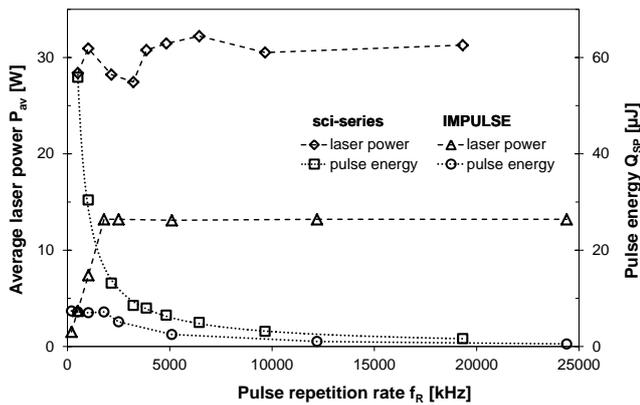
**Figure 4:** Average laser power and pulse energy versus repetition rate for both the *sci-series* and the *IMPULSE<sup>TM</sup>* laser.
