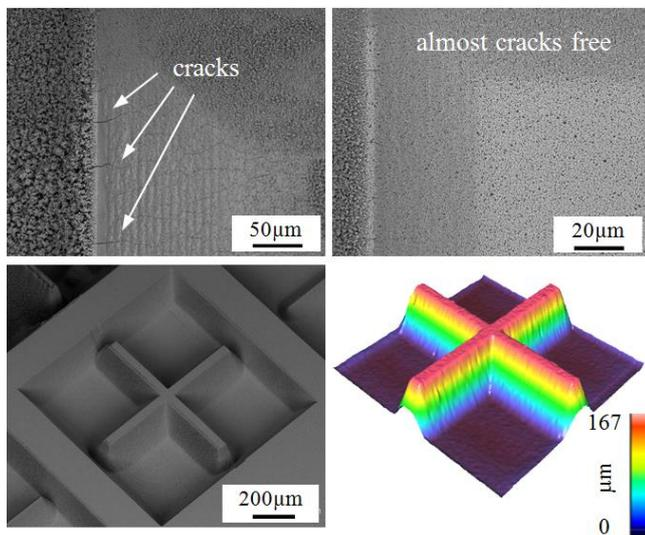
**Figure 10 top:** SEM images of wall edges obtained on zirconium oxide TZ-black with 5.9  $\mu\text{J}$  at 1.02 MHz and either 1  $\mu\text{m}$  (left) or 2  $\mu\text{m}$  (right) pulse spacing, micro cracks can be seen in the left picture; **bottom:** Demonstrator structure in zirconium oxide TZ-Black presented as SEM photograph (left) and 3D measurement (right).
