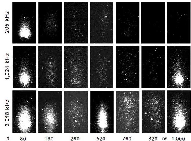
**Figure 3:** Ablation plumes arising on stainless steel upon femtosecond laser irradiation, pulse energy was 6  $\mu\text{J}$ ; recording times after the onset of the laser pulse are given in nanoseconds.
