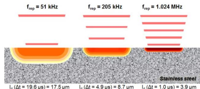
**Figure 1:** Heat affected volume illustrated for stainless steel and different repetition rates; heat diffusion lengths  $l_d$  are presented.
