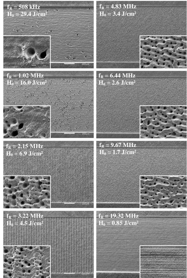
**Figure 13:** SEM photographs of laser processed cavity surfaces obtained with increasing repetition rates and decreasing fluence, respectively; cavity width was 1 mm.
