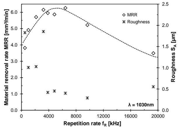
**Figure 7:** Material removal rate  $MRR$  and surface roughness  $S_a$  versus the repetition rate, obtained with a near-infrared laser beam of 31.7 W maximum average laser powers.
