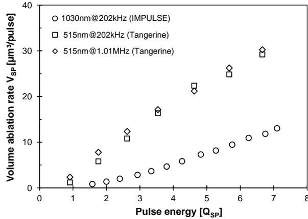
**Figure 4:** Volume ablation rate  $V_{SP}$  versus pulse energy  $Q_P$  presented for pulses of different wavelength and repetition rate.
