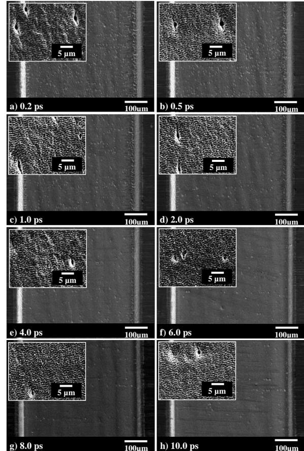
**Figure 10:** SEM micrographs showing the bottom of laser processed cavities over the edge to the unprocessed area; the cavities were produced with near-infrared laser pulses of 2.0 J/cm<sup>2</sup> fluence, 1.0 MHz repetition rate, and increasing pulse duration.
