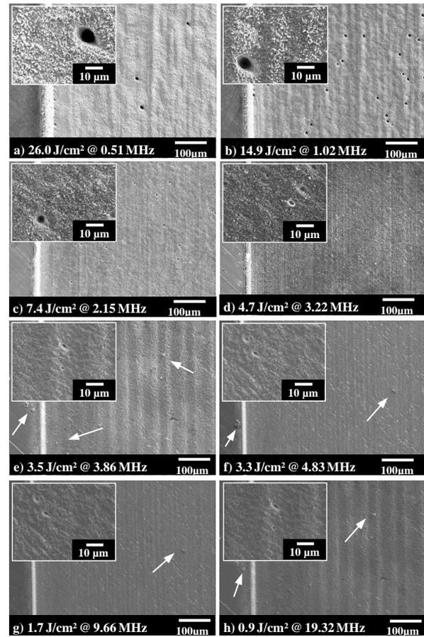
**Figure 8:** SEM micrographs showing the bottom of laser processed cavities over the edge to the unprocessed area, the cavities were produced with full available laser power of 31.7 W by varying the pulse repetition rate and respective the fluence.
