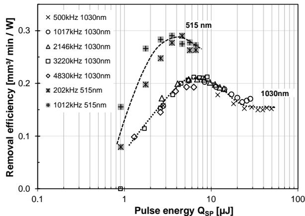
**Figure 5:** Material removal efficiency versus pulse energy  $Q_{SP}$ , presented for pulses of varied wavelength and repetition rate.
