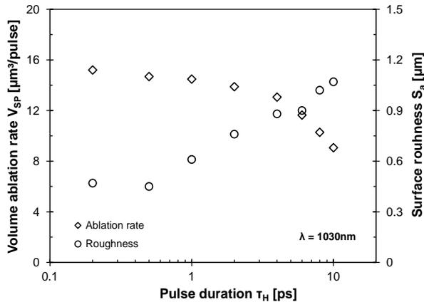
**Figure 9:** Volume ablation rate  $V_{SP}$  and surface roughness  $S_a$  versus pulse duration, obtained with near-infrared laser pulses of 2.0 J/cm<sup>2</sup> fluence and 1.0 MHz repetition rate.
