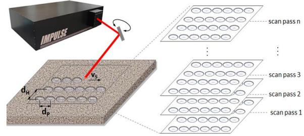
**Figure 2:** Sketch of the raster-scan processing regime where  $d_P$  is the pulse spacing,  $d_H$  is the hatch distance, and  $v_S$  is the scan speed.
