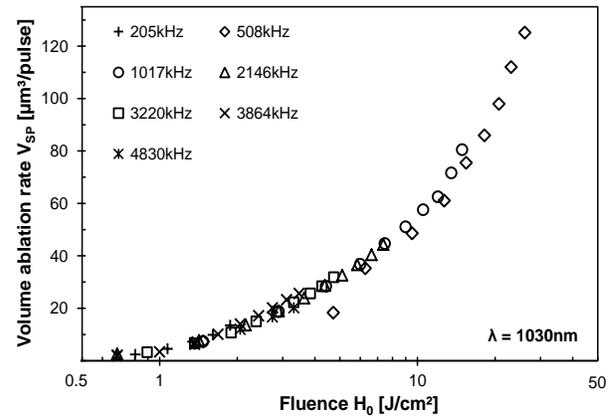
**Figure 6:** Volume ablation rate  $V_{SP}$  versus fluence  $H_0$ , obtained with near-infrared pulses of varied repetition rate in the range between 205 kHz and 4.8 MHz.
