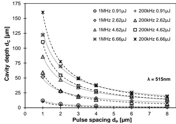
**Figure 3:** Cavity depth  $d_C$  versus pulse spacing  $d_P$ , obtained with pulses of varying repetition rate and energy; the wavelength was 515 nm.
