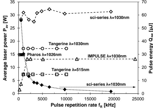
**Figure 1:** Average laser power  $P_{av}$  (on target) versus pulse repetition rate  $f_R$  presented for the used ultrashort pulse laser systems; the relation between pulse energy  $Q_{SP}$  and repetition rate is shown exemplarily for the *sci-series* laser.
