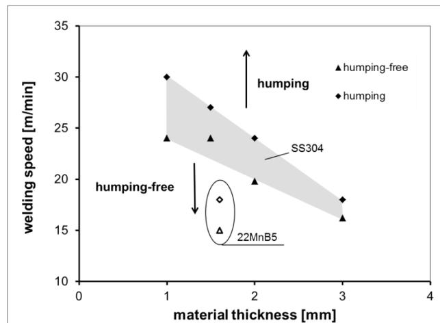
Figure 6: Maximum welding speed as a function of sheet thicknesses for SS304 and 22MnB5 for bead-on-plate welds, parameter:  $d_{86} = 65 \mu\text{m}$ .
