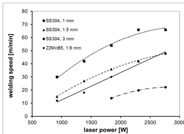
Figure 3: Maximum welding speed for SS304 and 22MnB5 as a function of laser power for bead-on-plate welds with different sheet thicknesses, parameter:  $d_{86} = 65 \mu\text{m}$ .
