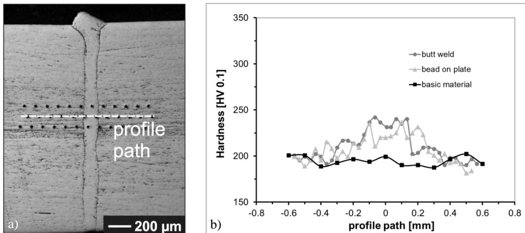
Figure 11: a) cross-section photograph of a butt weld, parameters:  $P_{cw} = 1840 \text{ W}$ ;  $v = 18 \text{ m/min}$ ;  $d_{86} = 53 \mu\text{m}$ ; SS304; b) corresponding hardness profile.
