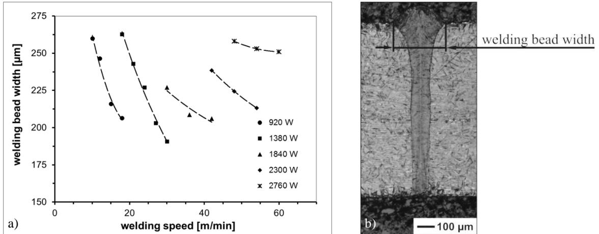
Figure 7: a) welding bead width as a function of welding speed and laser power, parameters: SS304, sheet thickness 1.5 mm; b) cross section photograph of a typical weld seam with nail-shaped head, parameters:  $P_{cw} = 920$  W,  $v = 18$  m/min,  $d_{86} = 65$  µm; SS304; sheet thickness 1mm.
