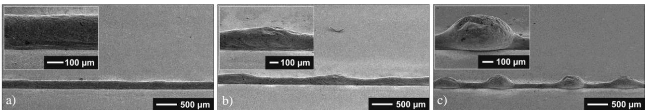
Figure 4: Humping formation for SS304 weld seams, parameters:  $P_{cw} = 1380 \text{ W}$ ; sheet thickness 1.5 mm; a) homogeneous humping-free seam,  $v = 24 \text{ m/min}$ ; b) incipient humping,  $v = 27 \text{ m/min}$ ; c) humping,  $v = 36 \text{ m/min}$ .
