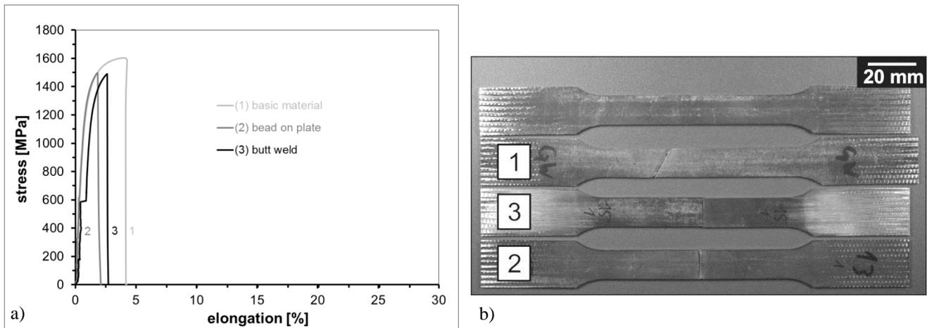
Figure 14: Tensile test results performed with 22MnB5 samples; a) stress-strain-curve; b) samples: (1) basic material, (2) bead-on-plate weld, (3) butt weld.
