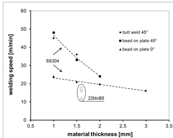
Figure 10: Welding speed as a function of material thickness depending on material and angle of incidence for bead-on-plate welds and butt welds, parameter:  $d_{86} = 53 \mu\text{m}$ .
