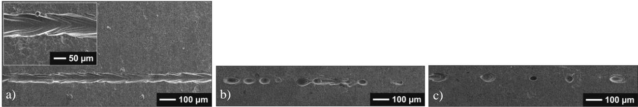
Figure 5: Spiking formation on SS304 weld roots, parameters:  $P_{cw} = 1380 \text{ W}$ ; sheet thickness 1.5 mm; a) homogeneously formed root,  $v = 27 \text{ m/min}$ ; b) non-uniform root formation indicates incipient spiking;  $v = 30 \text{ m/min}$ ; c) spiking,  $v = 33 \text{ m/min}$ ).
