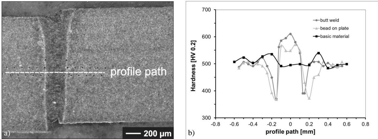
Figure 12: a) cross-section photograph of a butt weld, parameters:  $P_{cw} = 1840$  W;  $v = 16$  m/min;  $d_{86} = 53$  µm; 22MnB5; b) corresponding hardness profile.
