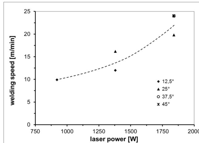
Figure 9: Maximum welding speed allowing humping- free weld seams as a function of the angle of incidence and laser power, parameters:  $d_{86} = 53 \mu\text{m}$ , sheet thickness 2mm, SS304.
