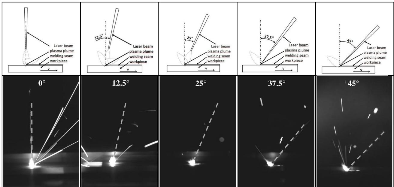
Figure 8: upper row) schematic drawings illustrating the angle of the incident laser beam and the preferred orientation of the plasma plume during welding, lower row) photographs of plasma plume formation during welding (dashed line: direction of incident laser beam), parameters:  $P_{cw} = 1.84$  kW,  $v = 18$  m/min,  $d_{86} = 53$  µm, SS304.
