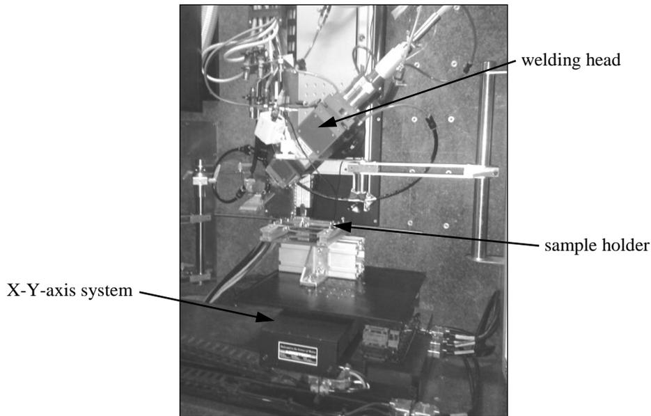
Figure 1: Experimental setup: tilted welding head, X-Y-axis system, sample holder.
