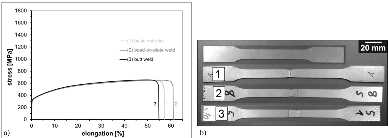
Figure 13: Tensile test results performed with SS304 samples, a) stress-strain-curve, b) samples: (1) basic material, (2) bead-on-plate weld, (3) butt weld.
