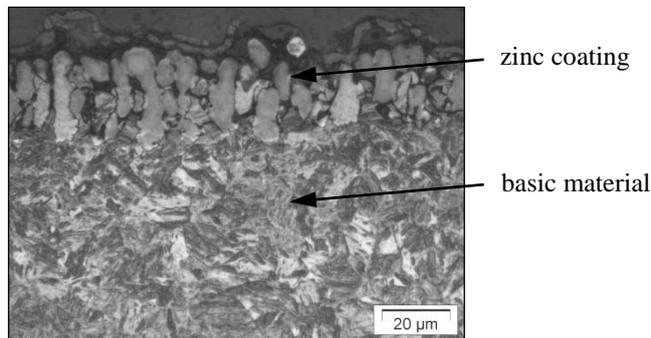
Figure 2: Cross-section photograph of 22MnB5: 20  $\mu\text{m}$  thick zinc coating on the steel surface is clearly visible.
